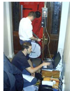
An airtightness test with the Blower-door equipment.
