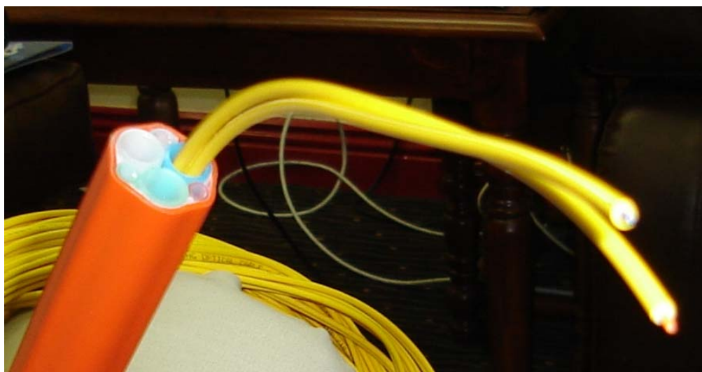
Figure 7 . An 8mm (ID) /10mm (OD) mini-tube housing two single fibres.
